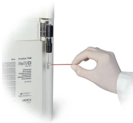
Self-contained Solutions Pack contains liquid calibrants and collects all waste, eliminates sample contact
